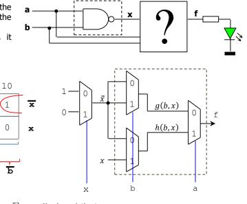
$f = xab + \bar{x}\bar{b} + \bar{x}\bar{a}$  $f(a, b, x) = \bar{a}f(0, b, x) + af(1, b, x) = \bar{a}(\bar{x} + \bar{x}\bar{b}) + a(xb + \bar{x}\bar{b}) = \bar{a}g(b, x) + ah(b, x)$  $g(b,x) = \bar{b}g(0,x) + bg(1,x) = \bar{b}(\bar{x}) + b(\bar{x})$  $h(b,x) = \overline{b}h(0,x) + bh(1,x) = \overline{b}(\overline{x}) + b(x)$ Also:  $\bar{x} = \bar{x}(1) + x(0)$
